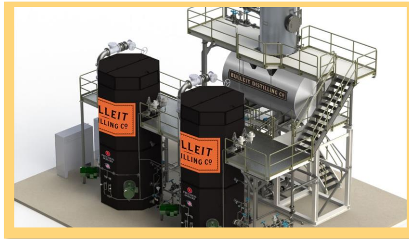
Figure 1.3: Rendering of electrode boilers to be installed at the Lebanon, Kentucky distillery. Courtesy of Precision Boiler and Diageo
